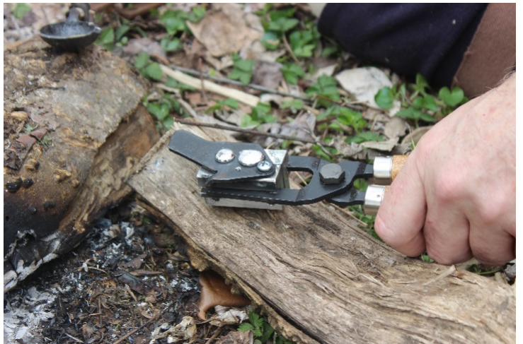
Lead is poured into the mold, this mold makes two bullets at a time.
