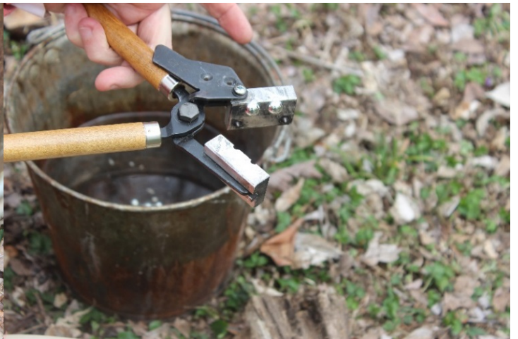
Shows bullets before being released from the mold
