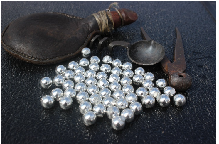
A perfectly round bullet will be more accurate. Carrying them in a bullet bag allows the balls to ride against each other and will help erase the sprue and the mold lines.
