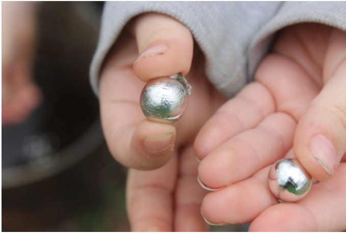
A finished bullet, note top where lead was poured into the mold – called the sprue. Also note a small line where the mold came together.
