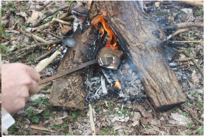
A ladle or pot can be used to melt lead
