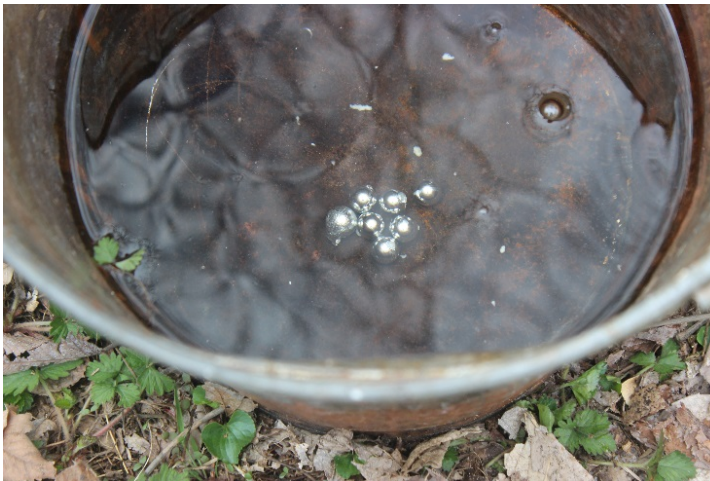
The bullets must be cooled before handling.
